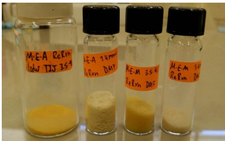
Figure S1. Physical appearance of the Mea , mea , Meb and meb resins, showing the characteristic yellow color of the conjugated aromatic Schiff base system
