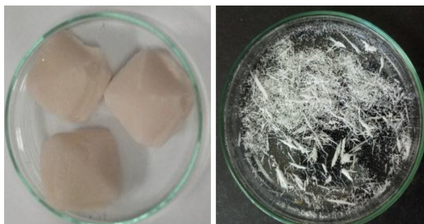
Figure 2. MA briquettes provided by the company Elekeiroz and MA obtained after crystallization in CHCl_3
