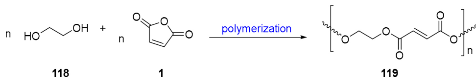
Scheme 47. Polymerization reaction of MA with ethylene glycol
