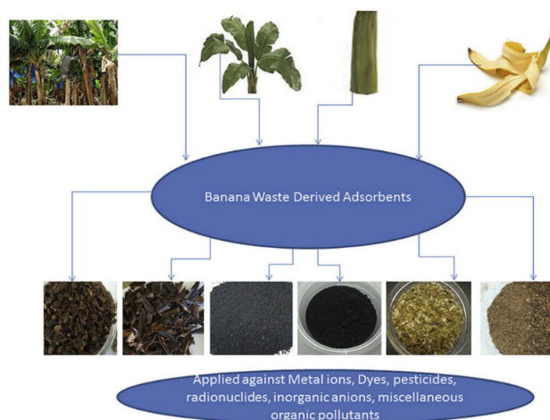
Figure 12. Different parts of banana tree applied to remove pollutants from water and wastewater. 234
