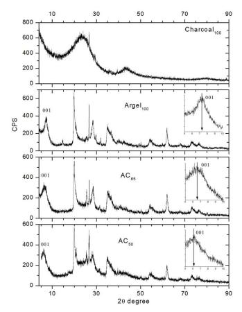
Figure 1. X-ray diffraction patterns of precursor's materials and composites:  $Charcoal_{100}$ ,  $Argel_{100}$ ,  $AC_{85}$  and  $AC_{50}$
