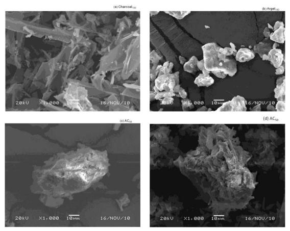
Figure 5. SEM images of the of precursor's materials and composites: Charcoal\_{100}, Argel\_{100}, AC\_{85} and AC\_{50}
