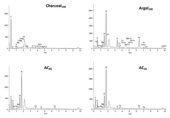
**Figure 3**. Chemical analysis by X-ray spectrometry energy dispersive (EDS) of precursor's materials and composites: Charcoal<sub>100</sub>, Argel<sub>100</sub>, AC<sub>85</sub> and AC<sub>50</sub>
