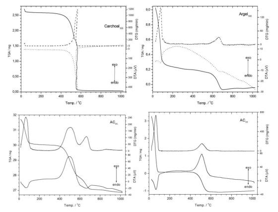
Figure 2. TG/DTA curves of precursor's materials and composites:  $Charcoal_{100}$ ,  $Argel_{100}$ ,  $AC_{85}$ and  $AC_{50}$
