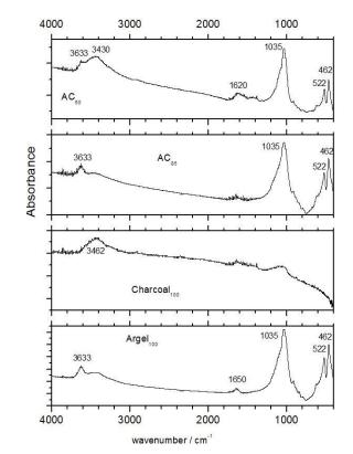
Figure 4. Vibrational spectra in the infrared region for the precursor's materials and composites:  $Charcoal_{100}$ ,  $Argel_{100}$ ,  $AC_{85}$  and  $AC_{50}$
