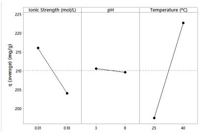
Figure 8. Graph for the interpretation of effects from  $2^3$  factorial design applied for the study of the methylene blue dye adsorption by AC<sub>50</sub> composite
