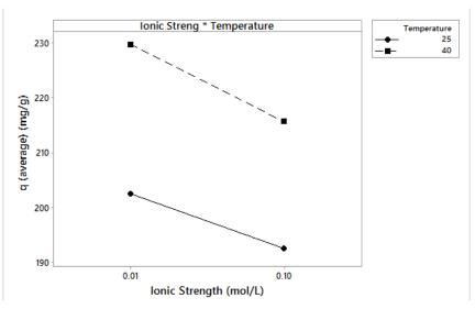
Figure 9. Graph of the interaction effect between ionic strength and temperature
