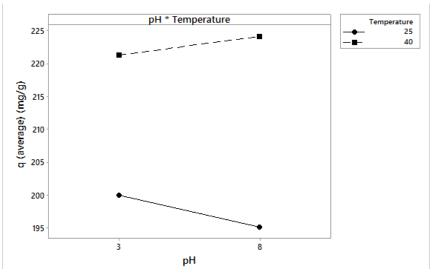
Figure 10. Graph of the interaction effect between pH and temperature.
