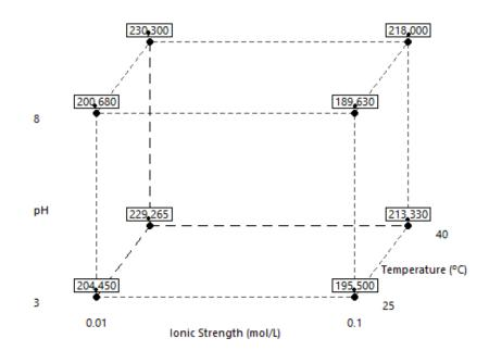
**Figure 11**. Interaction effect between temperature, pH and ionic strength for adsorption of methylene blue by AC<sub>50</sub> composite
