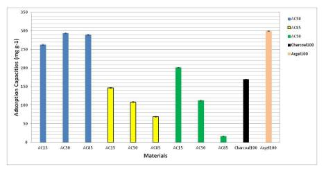
Figure 6. Comparison of the adsorption of metlhylene blue by the clay/coal composites
