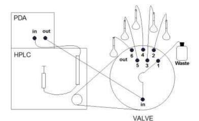
**Figure 2**. Flavonoids collection schema. Channel 1: waste reservoir; channel 2-5: flavonoid 2-5 reservoir; channel 6: flavonoid 6 or 7 (Source: own file)
