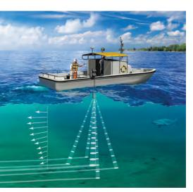
**Upgrade and Save**. Good news for RiverSurveyor M9 users who also require bathymetric data. Now you can upgrade your RiverSurveyor M9 to include the bathymetry power of the **HydroSurveyor** - a system designed to collect bathymetric, water column velocity profile, and acoustic bottom tracking data as part of a hydrographic survey.
